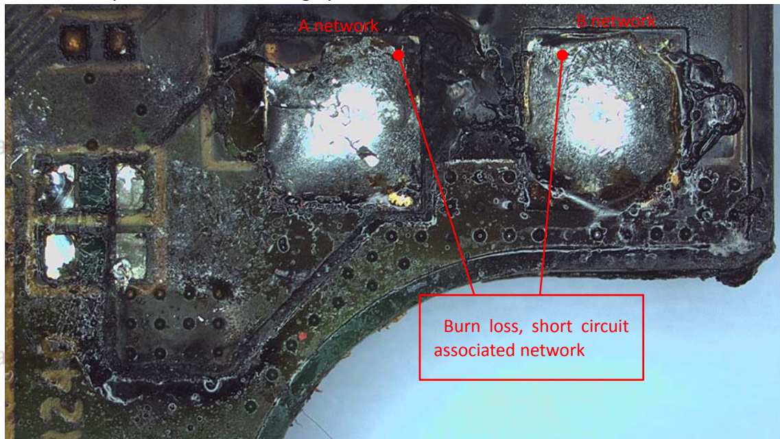
Observation picture of burn damage position on Bottom surface
